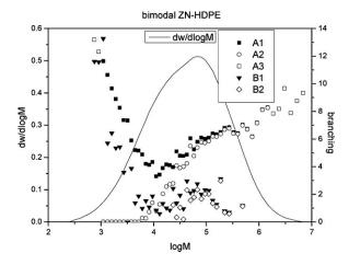
Figure 3. SEC-FTIR and SEC-IR analysis of a bimodal ZN-HDPE; methods A1 = OP < 0.96,  $CH_3/1000TC$ ; A2 = OP < 0.96, SCB/1000TC; A3 = OP > 0.96,  $CH_3/1000TC$ ;  $B1 = CH_3/1000TC$ ; B2 = SCB/1000TC.
