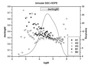
Figure 4. SEC-FTIR and SEC-IR analysis of a bimodal SSC-HDPE; methods A1 = OP < 0.96, CH<sub>3</sub>/1000TC; A2 = OP < 0.96, SCB/1000TC; A3 = OP > 0.96, CH<sub>3</sub>/1000TC; B1 = CH<sub>3</sub>/1000TC; B2 = SCB/1000TC.
