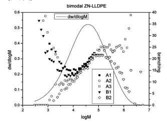
Figure 2. SEC-FTIR and SEC-IR analysis of a bimodal ZN-LLDPE; methods A1 = OP < 0.96, CH<sub>3</sub>/1000TC; A2 = OP < 0.96, SCB/1000TC; A3 = OP > 0.96, CH<sub>3</sub>/1000TC; B1 = CH<sub>3</sub>/1000TC; B2 = SCB/1000TC.
