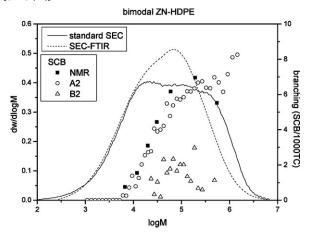
Figure 6. SEC, NMR, SEC-FTIR and SEC-IR analysis of a bimodal ZN-HDPE; methods A2 = OP < 0.96, SCB/1000TC; B2 = SCB/1000TC
