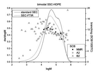
**Figure 7.** SEC, NMR, SEC-FTIR and SEC-IR analysis of a bimodal SSC-HDPE; methods A2 = OP < 0.96, SCB/1000TC; B2 = SCB/1000TC.
