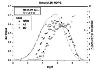
Figure 8. SEC, NMR, SEC-FTIR and SEC-IR analysis of a bimodal SSC-HDPE; methods A2 = OP < 0.96, SCB/1000TC; B3 = SCB/1000TC using dedicated calibration.
